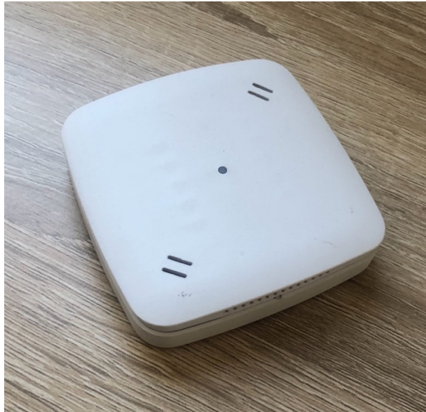
Figure 8. First tested case for Indoor Air Quality multi-sensor
